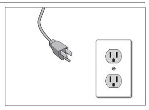
The EFX is for use on a nominal 120-volt circuit (refer to the WARNING below and to the *Installation Requirements* on page 2) and has a grounding plug that looks like the plug illustrated in Diagram A.
